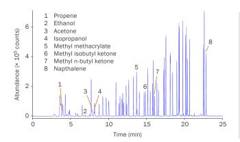
Use of the Kori-xr module with TT24-7xr provides excellent results for the analysis of a 100% RH, 65-component TO-15 standard containing polar and non-polar analytes.
