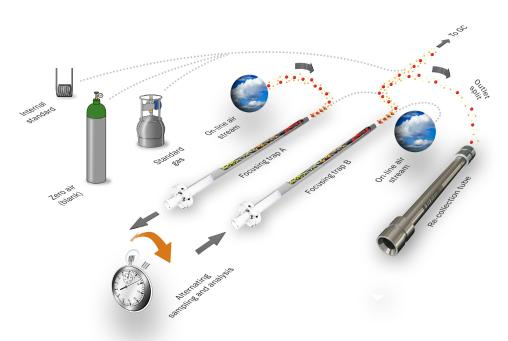
**Two focusing traps working in tandem** provide complete data-capture for on-line sampling of air using the TT24-7xr. At the time-point illustrated, sampling is taking place onto Trap A, while Trap B is being desorbed (with a portion of the flow to the GC being directed to a re-collection tube).
