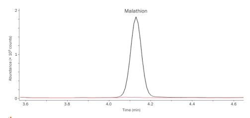
**Enhanced detection of low-volatility agents:** Quantitative recovery of higher-boiling, 'sticky' compounds like malathion (a VX simulant) with no carryover (red trace) is crucial for reliable trace-level measurements.
