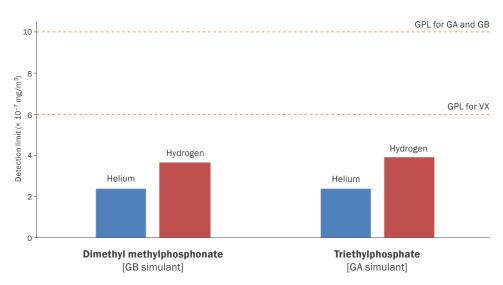
Ultra-sensitive, sub-GPL detection limits are achieved with both helium and hydrogen carrier gases, comfortably meeting even the most stringent reporting requirements with either gas.
