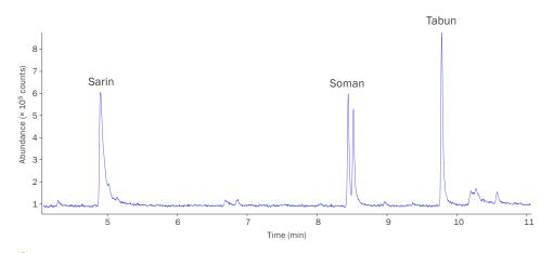
**Targeted measurement:** TT24-7NRT can be paired with selective GC-FPD for highly sensitive measurement of G agents, V agents and sulfur mustard.
