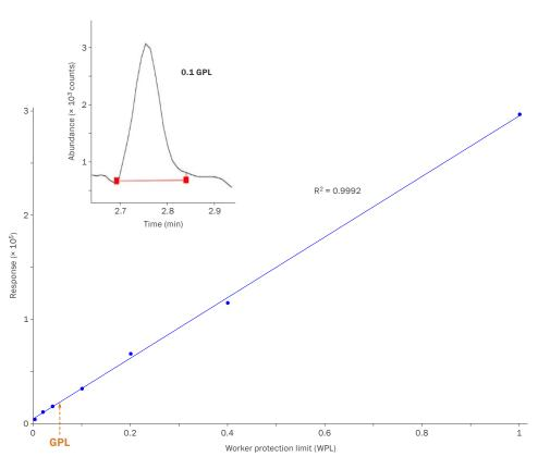
Linear calibration below the WPL for a sulfur mustard simulant (methyl salicylate) demonstrates limits of detection below even GPL levels. The extracted-ion chromatogram (inset) shows a quantifiable peak at 10% of the GPL (2  $\times$  10 $^{-6}$  mg/m³).
