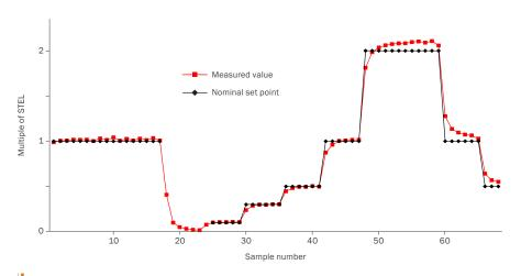
$\label{lem:concentrations} \mbox{ Airborne concentrations of sarin are closely tracked using tandem trapping for continuous monitoring of a generated atmosphere.}$
