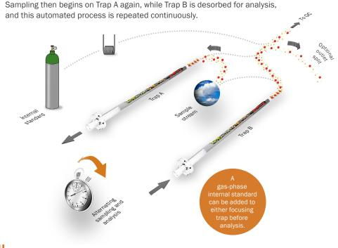
Operation of the TT24-7NRT. At the time-point shown, sampling is taking place onto Trap A, while Trap B is being desorbed.
