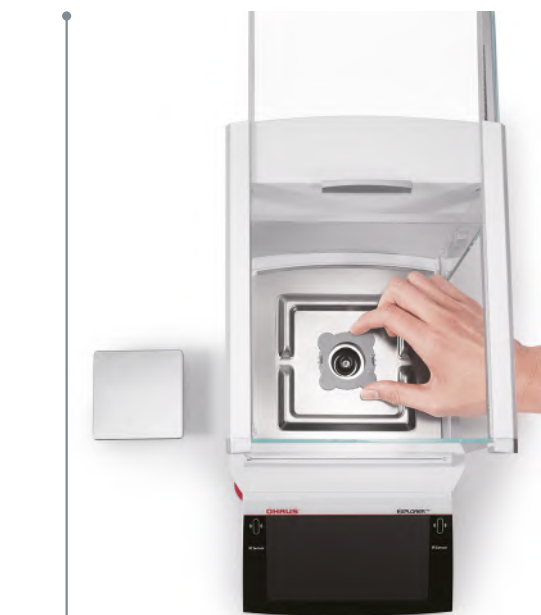
1 Unlock the draftshield fixed ring
