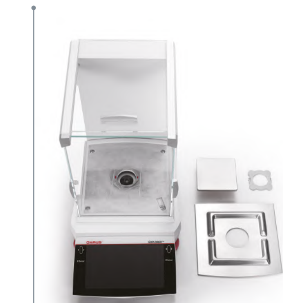
2 Remove EMC plate
