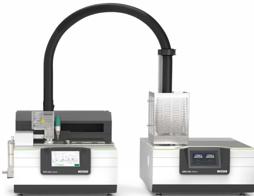
STA 319 Jupiter ® coupled to QMS 505 Aëolos ®
