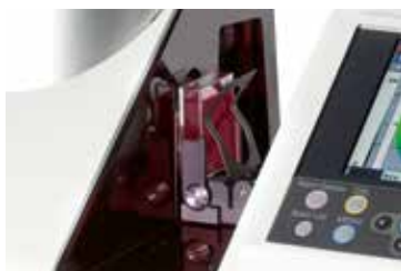
Measurement of liquids in transmission
