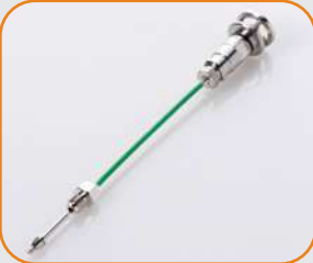
MODEL: 1260 11-3857 OEM G1367-87017 Needle Seat, 0.17mm ID, 0.8 mm OD, 600 bar
