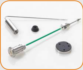
MODEL: 1100, 1200, 1120, 1220, 1260, G1313A, G1329A/B 11-4148 KIT OEM G1313-68719 PM Kit, G1329B • Seal, Pump (CTS-10621) 1 • Needle Assembly (CTS-10835) 1 • 2 Position/6 Port Rotor Seal, Vespel (600 bar) (CTS-12012) 1 • Needle Seat, Std., PEEK, 0.17mm ID (11-2605) 1
