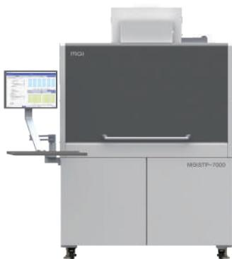
STP-7000 a high-throughput automated sample transfer processing system. It integrates tube decapping, tube recapping, barcode identification, automated liquid transfer and negative pressure protection. It decreases steps and delivers the quality and reliability you expect. You can transfer 192 samples from screw cap transport tubes or plain tubes to 96-Well Microplates in 40 minutes.
