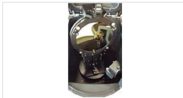
Figure 4. Front view of the Cary 7000 UMA sample compartment with the Agilent Solids Autosampler installed and the 200 mm diameter coated wafer mounted into the autosampler.
