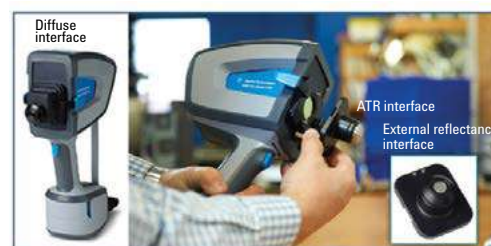
Figure 1. Agilent 4300 Handheld FTIR spectrometer with external reflectance (diffuse and specular) and internal reflectance (ATR) sampling interfaces. Interfaces can be changed in seconds, with no realignment required.
