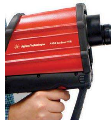
Figure 1. Agilent 4100 ExoScan FTIR spectrometer equipped with diffuse reflectance sample interface for measurement of composites
