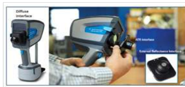
Figure 1. The Agilent 4300 hand held FTIR instrument, with the three interchangeable interfaces used in this study.
