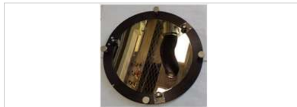
Figure 3. A 200 mm diameter precut wafer mounted in the 8" sample holder that attaches into the Solids Autosampler.
