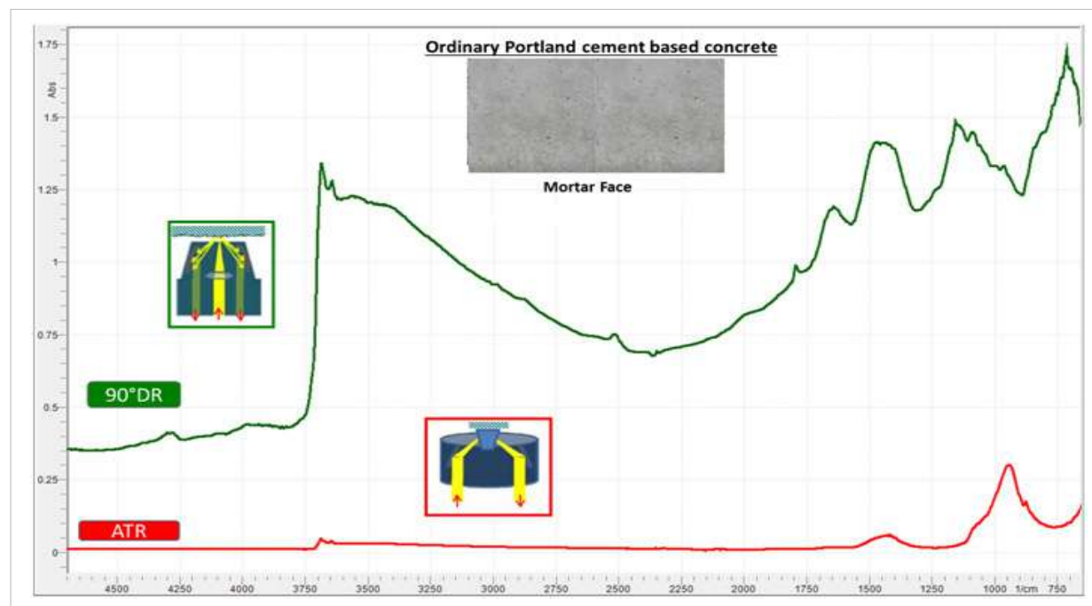
Figure 3. ATR spectra (red) of the powdered concrete and Diffuse Reflectance Spectra (green) of the mortar face of a concrete sample without any sample preparation.
