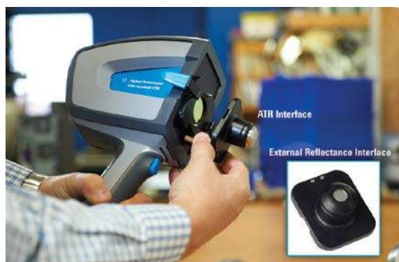
Figure 2. Agilent 4300 Handheld FTIR with diamond ATR and external reflectance sample interfaces used for measurement of PET. Sample interfaces are instantly interchangeable with no realignment necessary.
