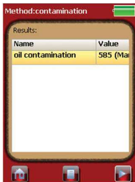
Figure 3. 4100 ExoScan FTIR Results screen showing a marginal oil contamination on a metal surface
