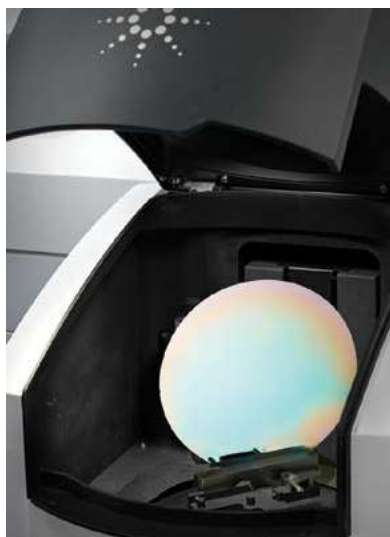
Figure 1. Agilent Cary 7000 UMS with a 200 mm diameter silicon wafer sample mounted in the measurement chamber
